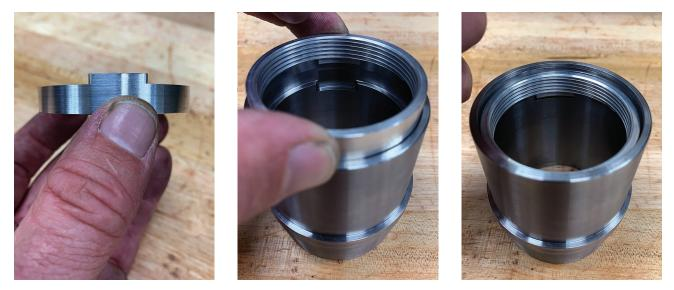
Figure 8: Installing the threaded aluminum ring into the steel weld in bump stop holders
