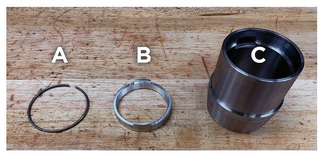
Figure 7: Bump Stop Holder Parts
