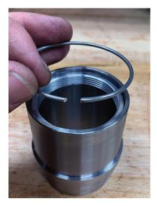
Figure 9: Installing the wire snap ring
